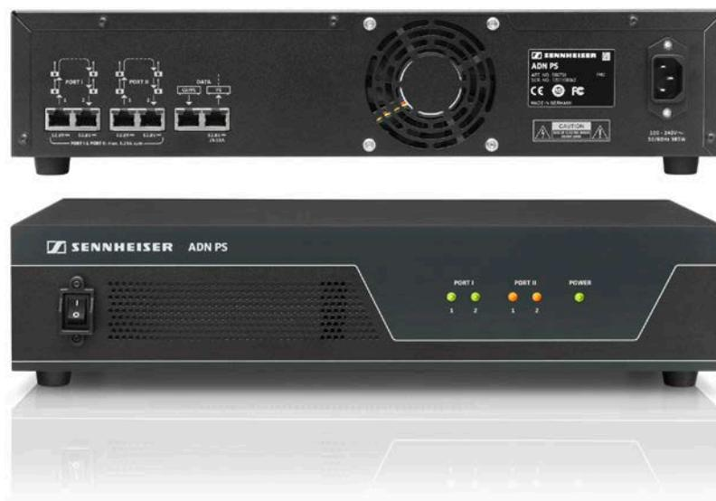
The cascadable ADN PS Power Supply allows the extension of up to 400 conference units to the ADN CU1 central unit. It also increases the failuresafety of the system by allowing redundant ring-cabling on its four conference ports. Up to 40 units can be connected in two rings and up to 70 units in alternative branch cabling. Status LEDs at the front of the 19" rack-mount unit indicate the type of cabling to easily monitor the system.
